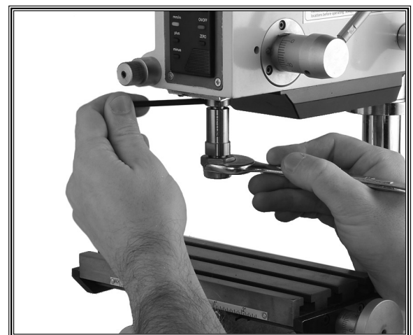
Figure 25. Installing a collet.
